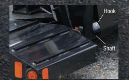
Hydraulic removable "shaft & hook" gooseneck is the fastest and most versatile in the industry–especially on uneven ground. Industry leading 12" deck height with 4" ground clearance.
